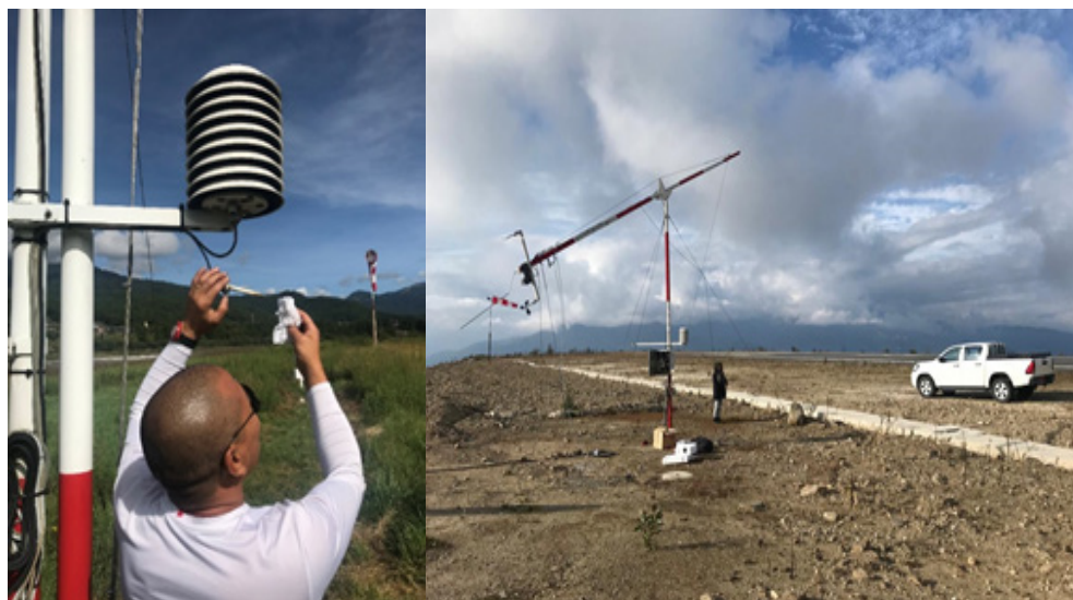
Figure 13: Cleaning of air temperature sensor (left) and replacing sensors of Yongphula AWOS (right)
