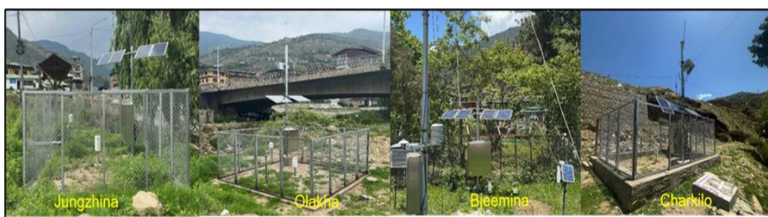
Figure 19: Automatic River Discharge Measurement Station established on the tributaries of the Thimchhu
