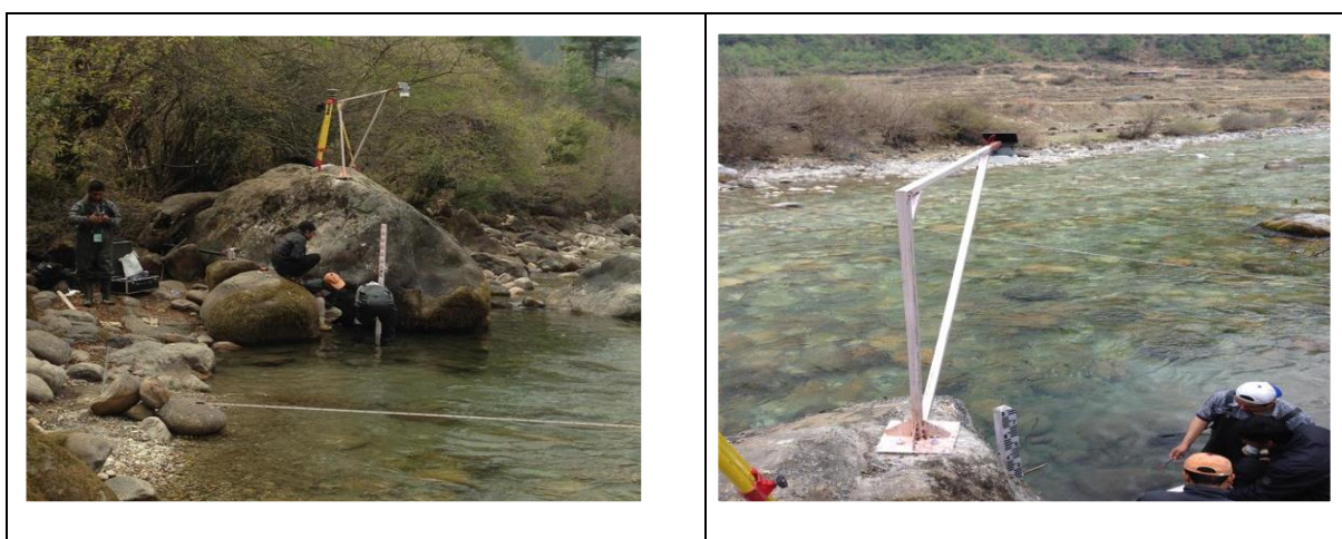
Figure 58: Mini Ultrasonic Water Level Sensors installed on Pachhu below Drukgyal Dzong.
