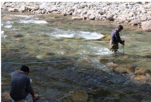
Figure 53: Discharge measurement of Pipingchhu
