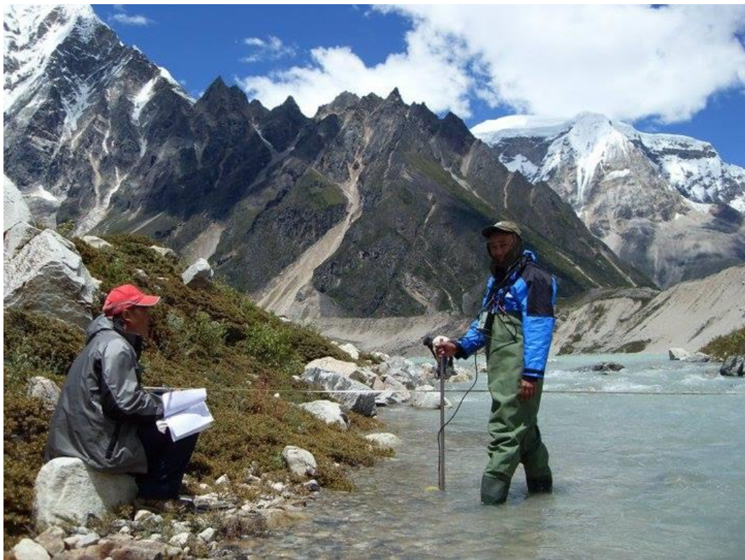
Flow measurement by Wading method in Lunana
