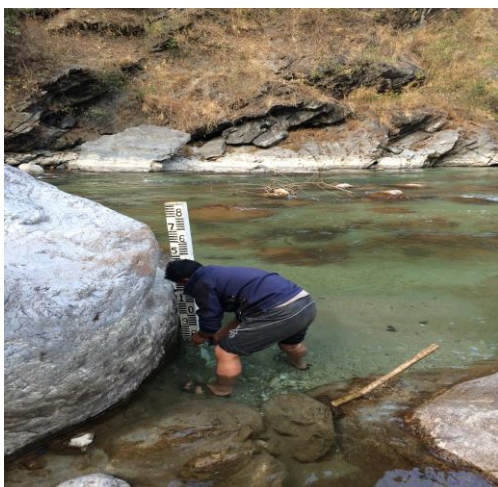
Figure 55: Technician installing river gauge post at Nyera Ama ri
