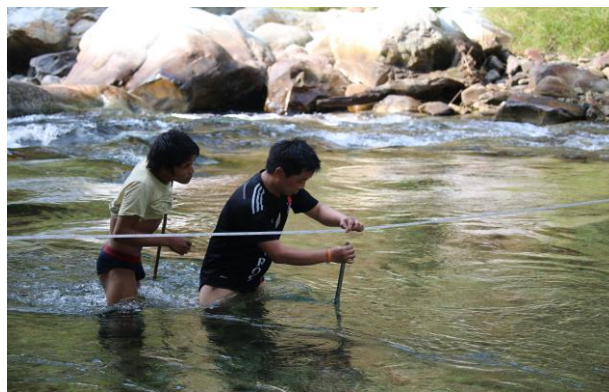
Figure 54: Hands on training of flow measurement imparted to local staff by Hydrology Division team.
