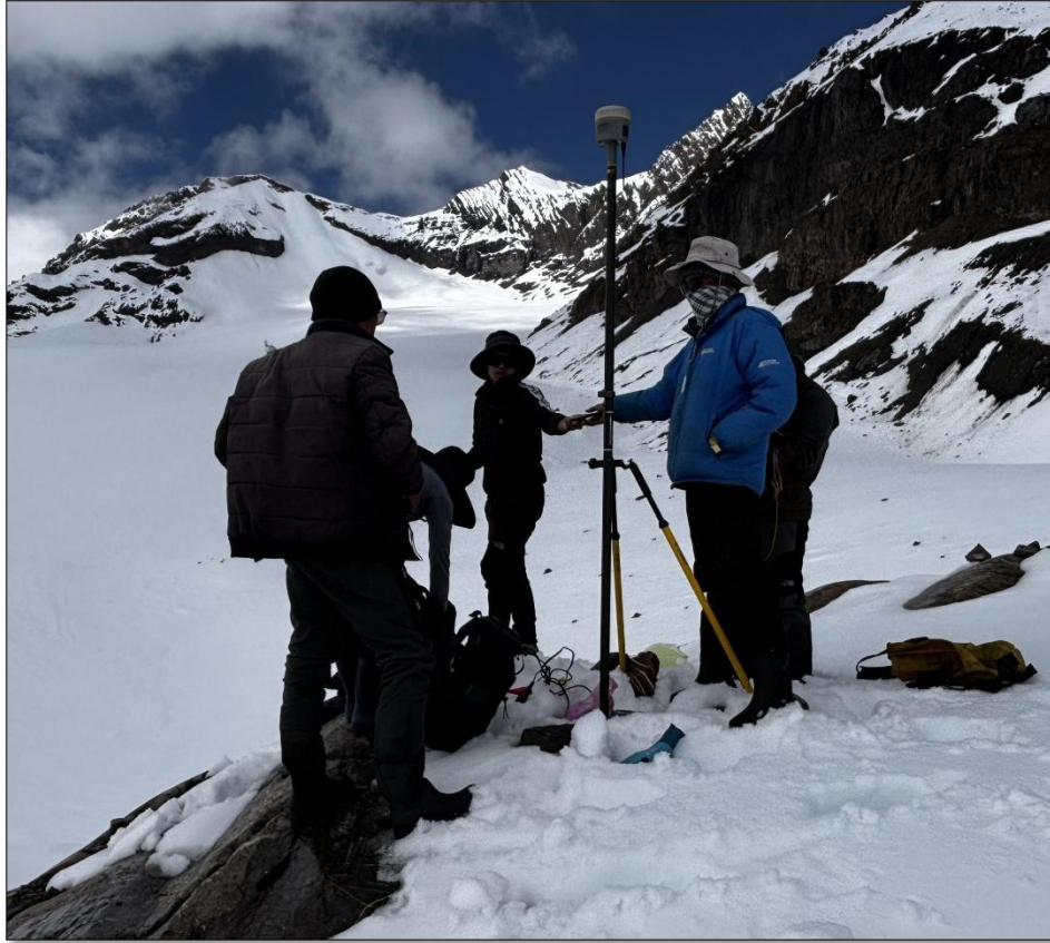
Figure 3. RTK GNSS base-station setup used during the field survey.
