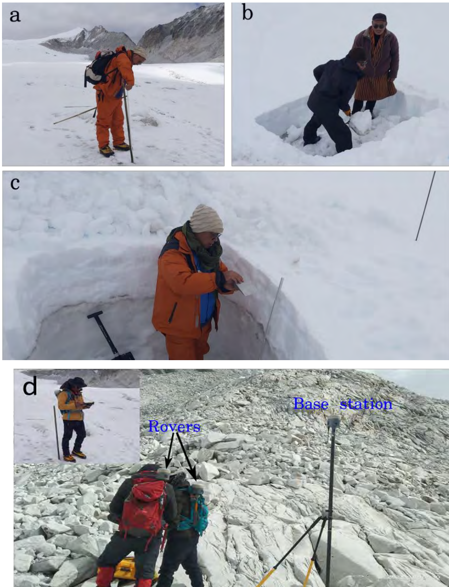
Figure 38:: a) Retrieval of old stakes, b&c) Snow-pit Measurement. d) Setting up of base for dGPS survey.
