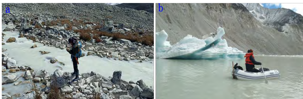
Figure 40: Figure showing topographical mapping at the outlet (a) and lake bathymetry survey (b)
