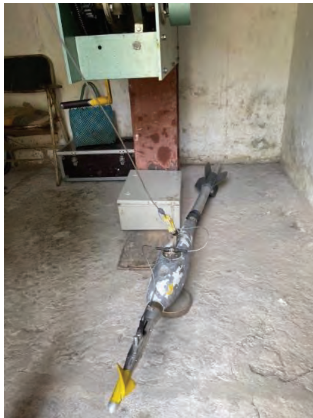
Figure 16. Example of a principal hydrological station and current meter in Thimphu
