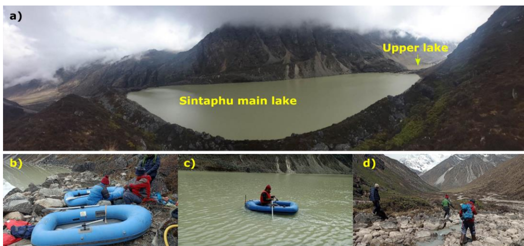
Figure 32: Field photos of Sintaphu Lake; a) Panoramic view of Sintaphu main lake and upper lake, b) Inflating rubber boats for bathymetry survey, c) Lake bathymetry survey, and d) moraine and outlet channel topography mapping using Trimble GNSS R10-2
