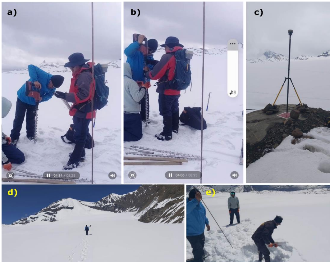
Figure 29: Field survey work on Shodug glacier, 2023. a & b) Drilling and installation of bamboo stakes on glacier surface, c) Trimble GNSS base station, c) walking on the glacier surface caring rover on backpack to map the glacier surface elevation and e) Snowpit measurement
