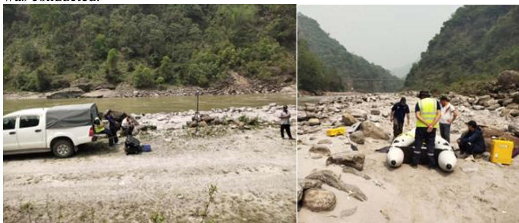
Figure 17: Field data collection for development of rating curve at Dorokha AWLS
