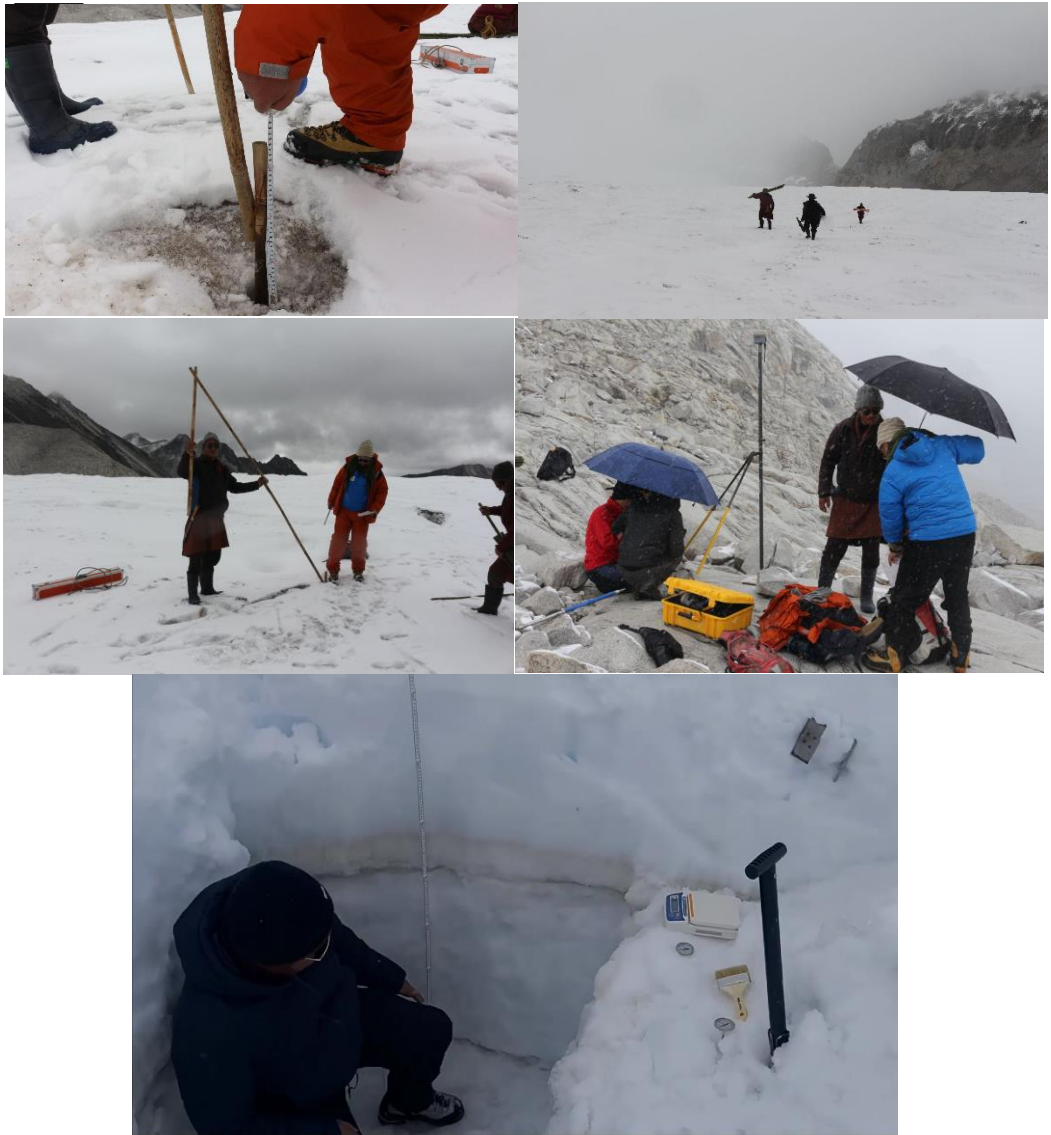
Figure 27: Retrieval of old stakes, Setting up of base for dGPS survey, Measuring old stakes above ice, Field survey works on Thana Glacier and Snow-pit Measurement.
