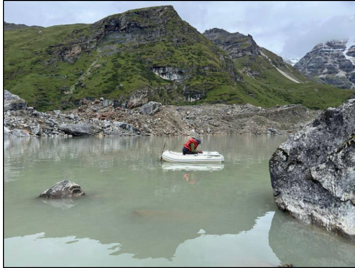
Figure 3. Bathymetric survey of Jechu Drake Lake using a SONAR/GPS-integrated sensor mounted on an inflatable survey boat.
