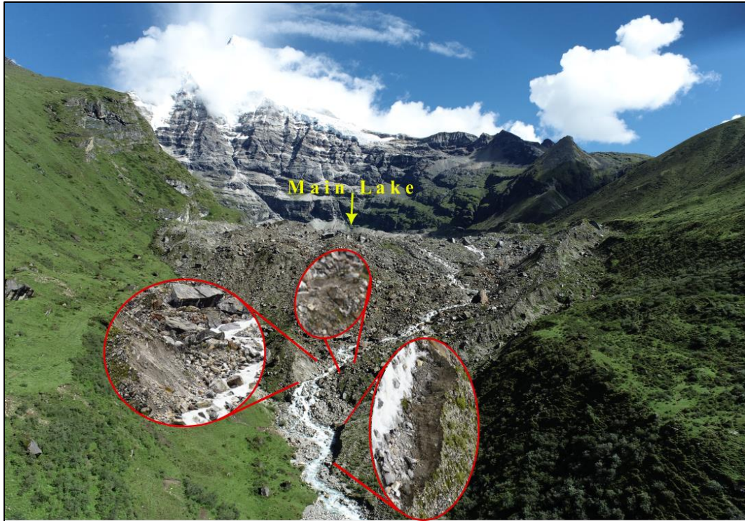
Figure 8. Localised scour zones observed at the foot of the main lake's damming moraine.
