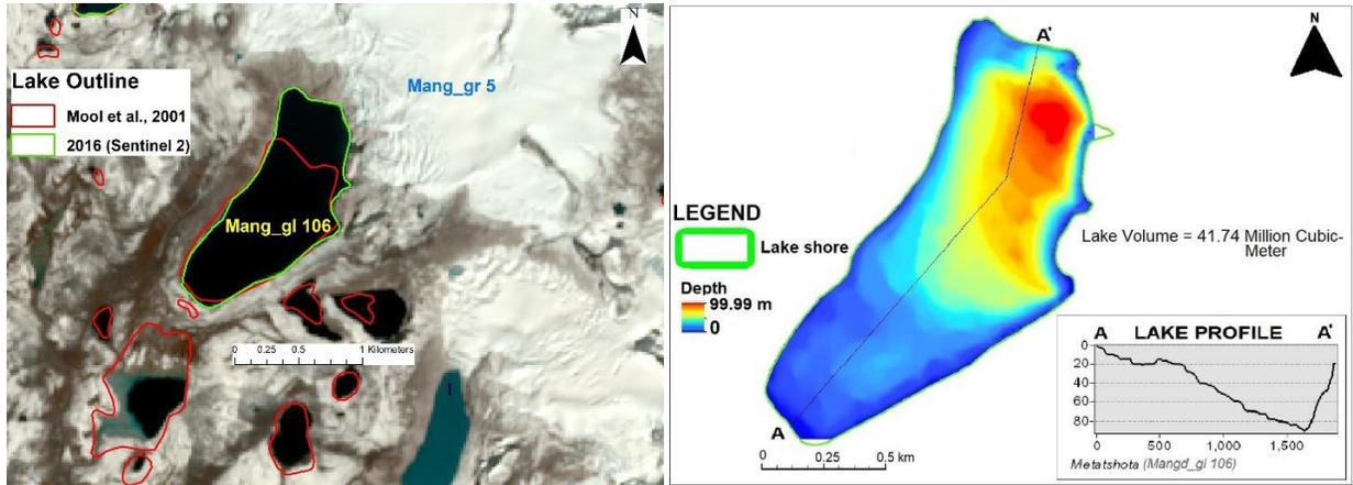
**Figure 3.17: Left:** Mang\_gl 106 (Metatshota) delineated using Sentinel 2 of 2016 (Green) IRS ID of 1999 (Mool et al., 2001). **Right:** Lake bathymetry map prepared using the data set of 2009 (DGM-JICA/JST GLOF Project) along with depth profile A-A'
