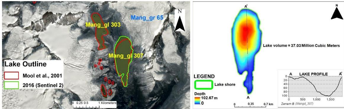
**Figure 3.21:** *Left:* Mang\_gl 307 (Zanam B) and Mang\_gl 303 (Zanam A) on Sentinel 2 (2016) imagery. The red polygon is the lake outlines by Mool et al., 2001 and green is from Sentinel 2 (2016). *Right:* Bathymetry map of Mang\_gl 307 along with depth profile from outlet to upper reach (A-A').
