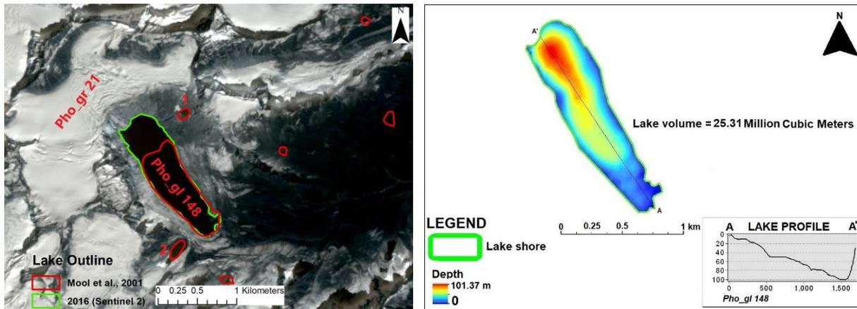
**Figure 3.7:** *Left: Pho\_gl 148 with adjacent lakes lying at higher elevation (1&2) and the feeding glacier Pho\_gr 21 which wastes part of it in the form of icefall into the lake. Green and the red polygon shows the lake outline of 2016 (Sentinel 2) and Mool et al., 2001 respectively. Background image is Sentinel 2 (2016). Right: Bathymetry map of the lake with depth profile (A-A'). Lake has shallow depth at the outlet part and deeper towards the upper reach.*
