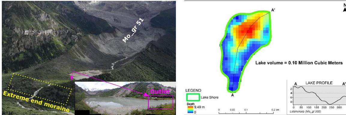
**Figure 3.4:** Left: Photo of Latshokarp show the location of Mo\_gr 51. The lake has a wide open outlet which is shown in pink rectangular box. Yellow dotted box shows the extreme end moraine. Right: Bathymetry map of the lake with the depth profiles A-A'.
