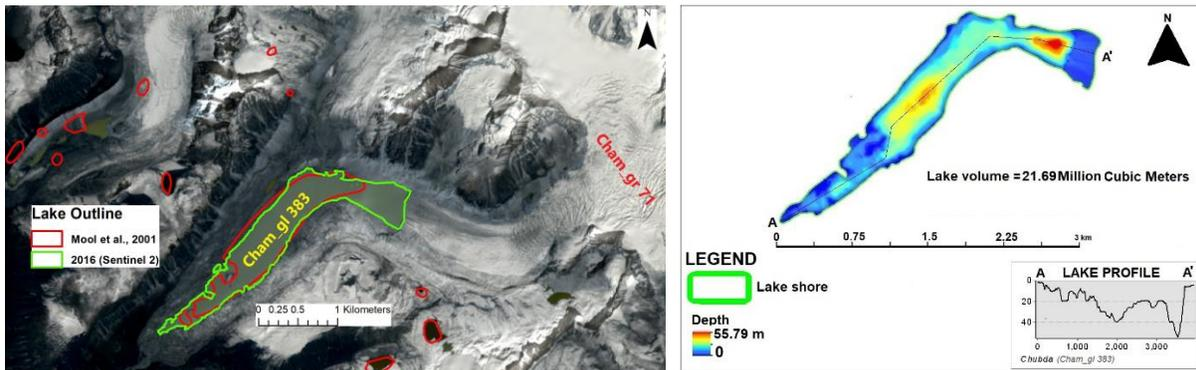
**Figure 3.27: Left:** Cham\_gl 383 (Chubda Tsho) on Sentinel 2 (2016) imagery. The red polygon is the lake outline by Mool et al., 2001 and green is from Sentinel 2 (2016). **Right:** Bathymetry map of Cham\_gl 383 along with depth profile from outlet to upper reach (A-A')
