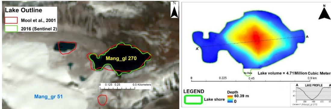
**Figure 3.19:** Left: Mang\_gl 207 (lake Zanam F) on Sentinel 2 (2016) image with lake polygons of Mool et al., 2016 (red) and Sentinel 2 (2016). Right: Lake bathymetry map with depth profile (A-A').
