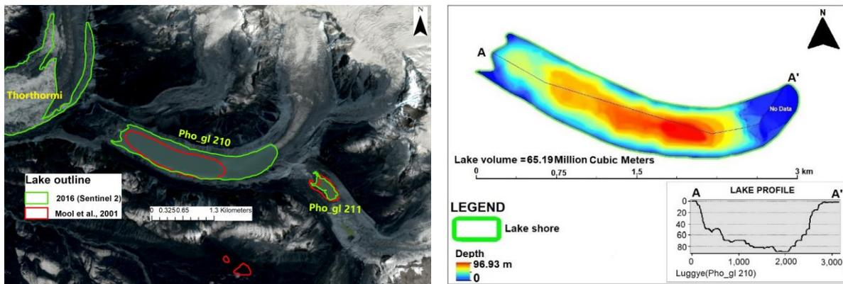
**Figure 3.13:** Left: Mo\_gl 210 (Lugge Tsho) on Sentinel 2 image. Green and red polygon are the Lake Outline from Sentinel 2 (2016) and Mool et al., 2001. Pho\_gl 211 is Drukchung lake. Right: Bathymetry map of Lugge lake (data from 2011). Due to lack of data coverage towards the upper reach, the depth interpolated is lesser.
