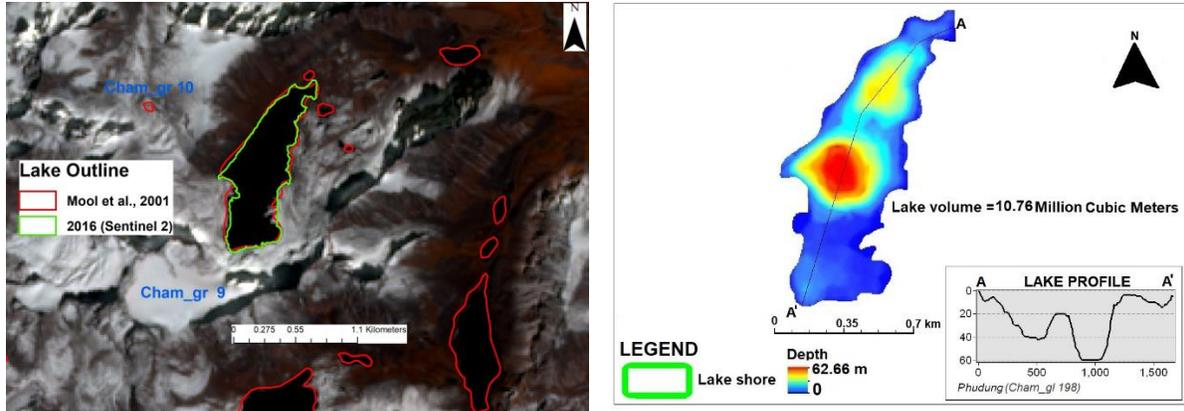
**Figure 3.24:** *Left:* Cham\_gl 198 (Phudung Tsho) on Sentinel 2 (2016) imagery. The red polygon is the lake outline by Mool et al., 2001 and green is from Sentinel 2 (2016). *Right:* Bathymetry map of Cham\_gl 198 along with depth profile from outlet to upper reach (A-A')
