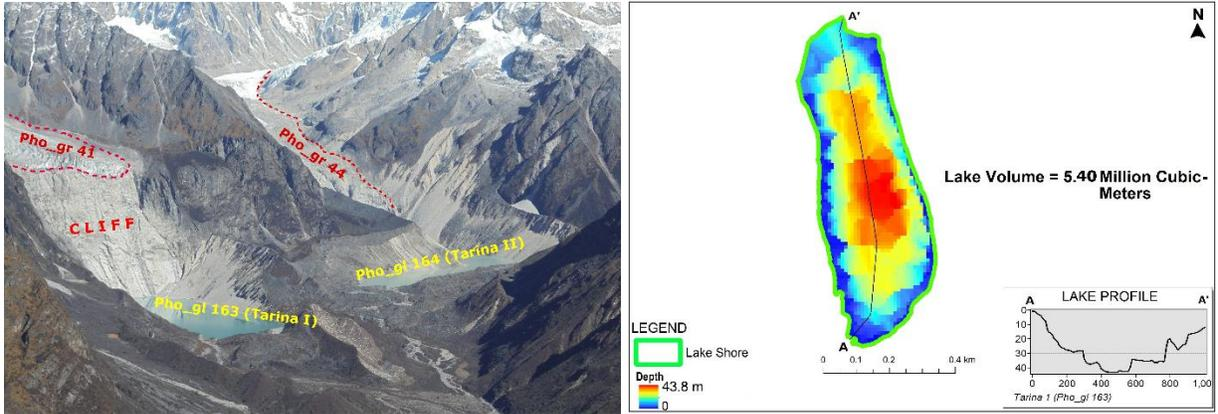
**Figure 3.8:** *Left: Photo showing Tarina I, Tarina II, Pho\_gr 41, Pho\_gr 44 and the Cliff along which the Pho\_gr 41 feeds Tarina I in the form of ice fall. Right: Bathymetry map of Tarina I along with the depth profile from the outlet towards upper reach of the lake (A-A')*
