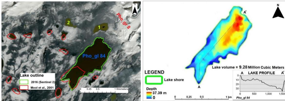
**Figure 3.6 :**Left: Pho\_gl 84 on Sentinel 2 (2016) with other adjacent lakes and feeding glacier Pho\_gr 8. Green and red polygons are the lake outline from Sentinel 2 and by Mool et al., 2001. Number 1 and 2 are the new lakes formed. Right: Bathymetry map of the lake with the depth profile A-A'
