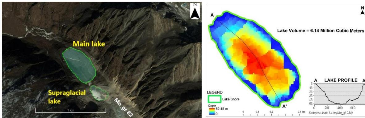
**Figure 3.5:** *Left: Sintaphu glacial lake and the supraglacial lake on google earth pro image (imagery date: 1-4-2014). The lake boundaries are from the Sentinel 2 image (2016). Right: Bathymetry map of the main lake with depth profile from outlet towards upper reach (A'-A)*
