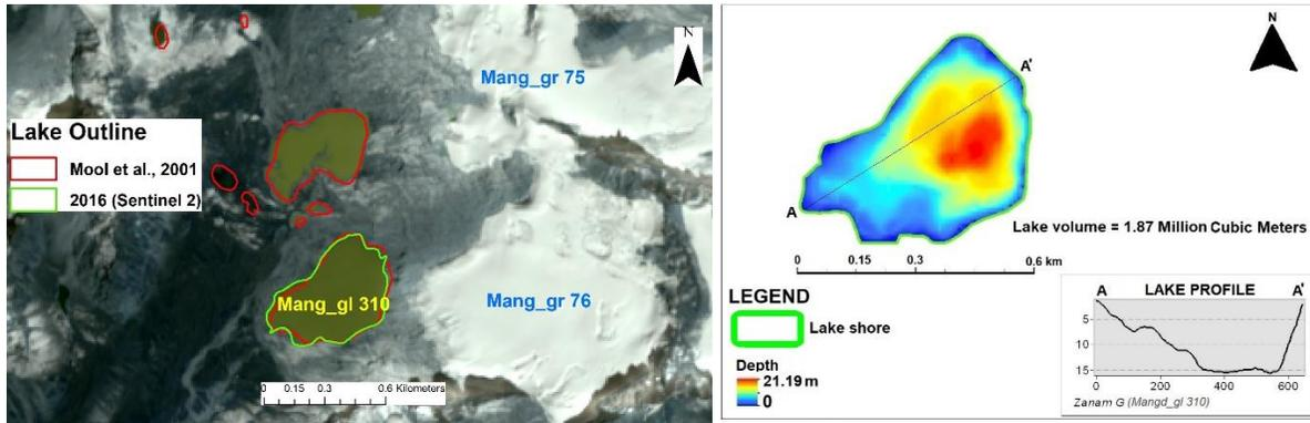
**Figure 3.22:** *Left:* Mang\_gl 310 (Zanam G) on Sentinel 2 (2016) imagery. The red polygon is the lake outline by Mool et al., 2001 and green is from Sentinel 2 (2016). **Right:** Bathymetry map of Mang\_gl 310 along with depth profile from outlet to upper reach (A-A').
