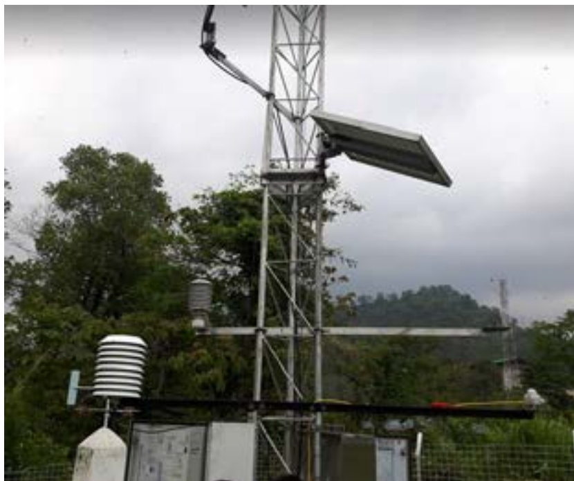
Figure 19: AWS at Rinchending with additional sensors and accessories from MICROSTEP
